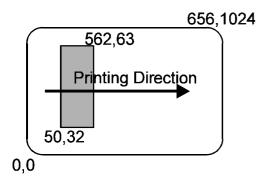
With the ESC-Sequence 'Data Transmission' image data may be transmitted to the printer or image storage partially deleted. The respective operation mode is set by the modus ('L' =Delete) and 'S' = Write. The data are transmitted line wise (X-direction) to the printer. In Illustration 1, Coordinate System TOP-ino Printer, the coordinate system used by the printer is demonstrated. By setting the X- and Y-start position, entering image data may be started at any location in the image storage
