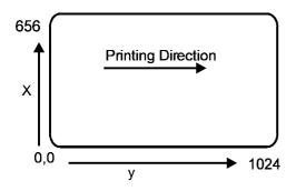
The printer may print a maximum of 656 X 1024 pixel. This way, a plastic card of the format 54mm X 86mm may be printed completely. In the edge area 2-4 pixel may be printer externally of the card. This way, tolerances of the various cards may be evened out.
