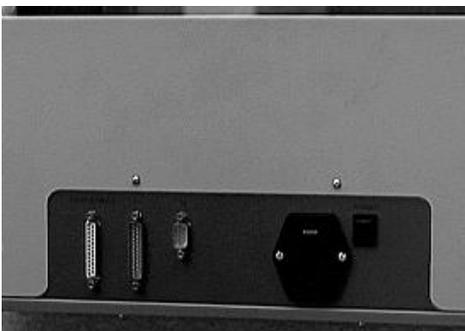
This serial interface is used for remote control. Here it is possible to control and supervise the complete print technical process by using a terminal (i.e. Win 3.11, accessories, terminal, 9600 b/s or Win 95 with the hyperterminal). The main functions are password secured.
